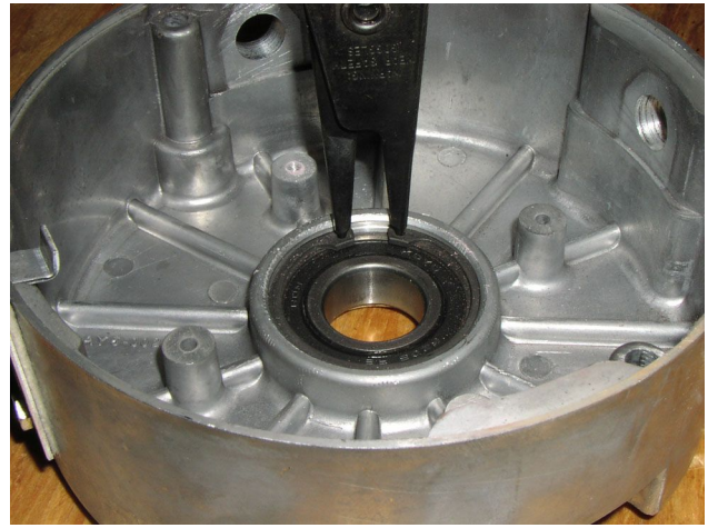
Figure 16-11 Bearing Retaining Ring
