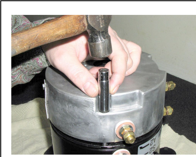
Figure 16-6 End Cap Disengagement
