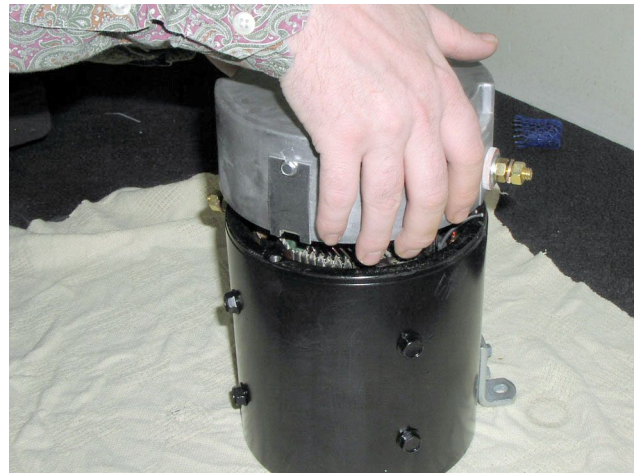
Figure 16-7 End Cap Removal
