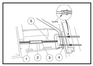
Figure 6-19 Loosen Brake Cables
