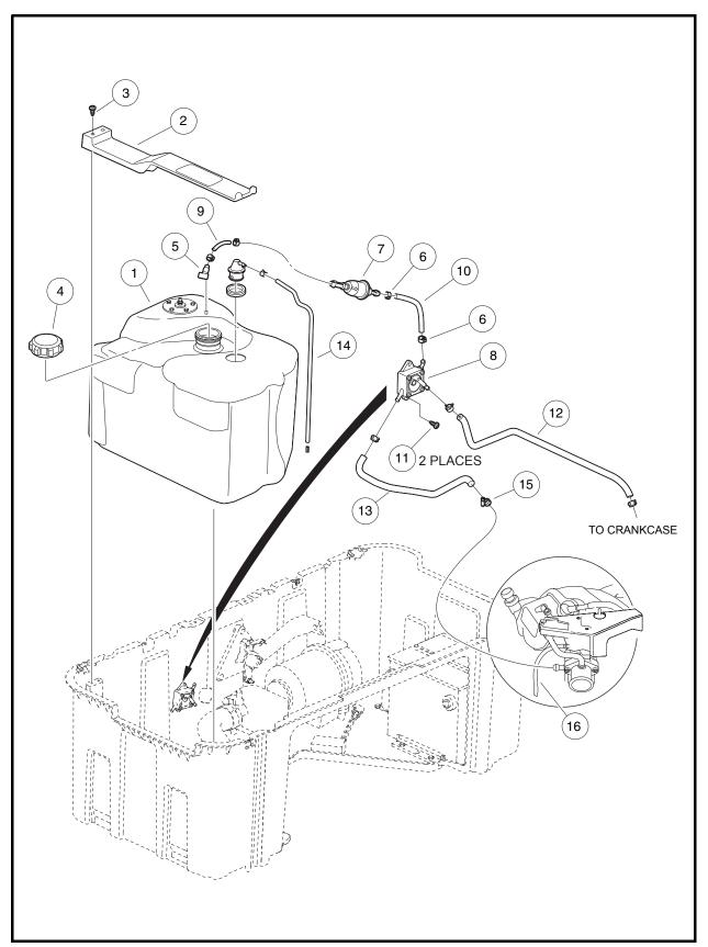
Figure 14-8 Fuel and Vent Lines
