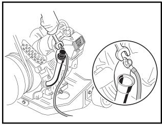
Figure 16-48 Connect Shifter Cable
