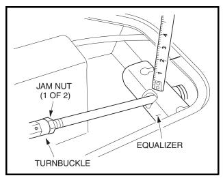
Figure 6-18 Brake Equalizer Adjustment
