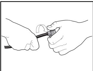
Figure 11-28 Spark Plug Cap Removal
