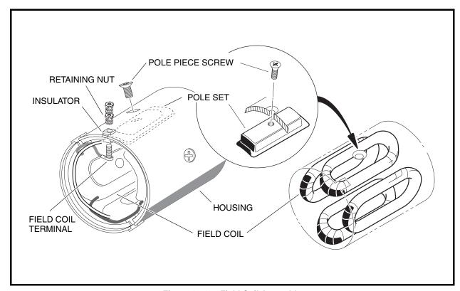
Figure 12-10 Field Coil Assembly
