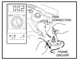
Figure 11-12 Fuel Tank Ground
