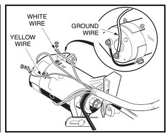
Figure 16-16 Generator Wires
