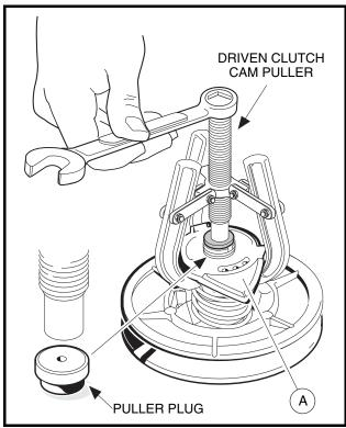
Figure 17-21 Driven Clutch Disassembly
