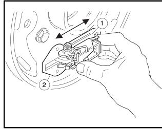
Figure 6-8 Lubricate Slide and Slide Plate
