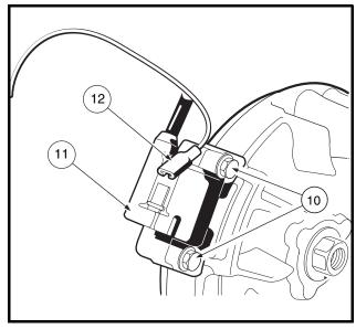
Figure 12-27 Fan Housing and Shroud Installation
