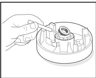
Figure 17-15 Spiral Back-up Rings
