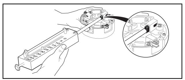
Figure 12-5 Brush Spring Tension Test
