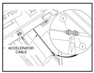
Figure 5-9 Accelerator Cable Adjustments
