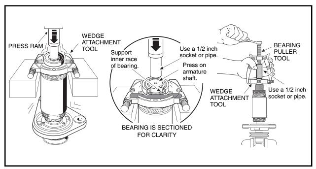
Figure 12-9 Bearing Removal
