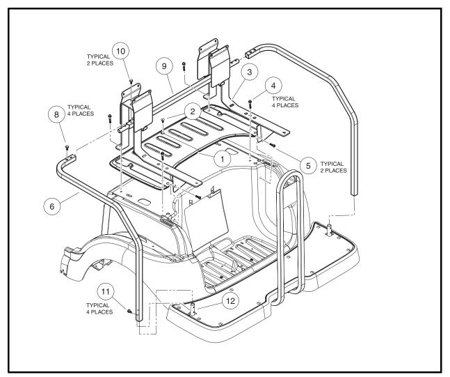
Figure 4-9 Seat Supports (Four-Passenger Vehicles)
