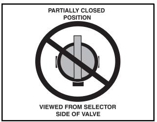
Figure 3-5 Incorrect Fuel Shut-off Valve Setting
