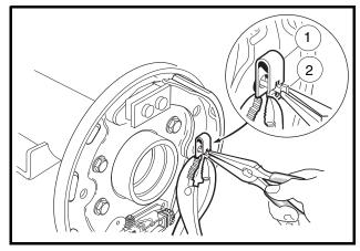
Figure 6-13 Install Trailing Shoe Retainer Clip
