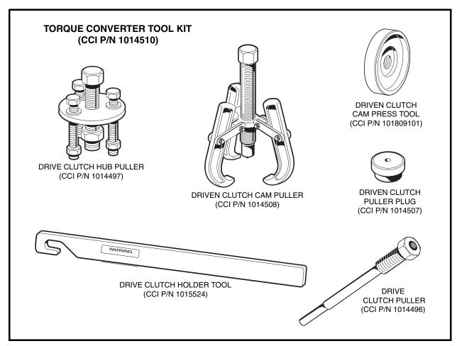
Figure 17-1 Torque Converter Tool Kit
