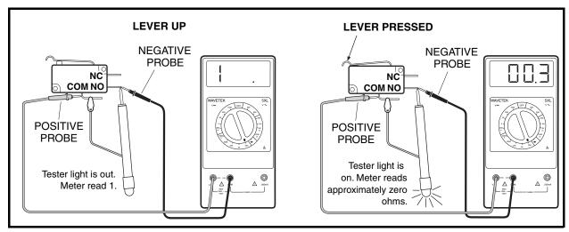
Figure 11-18 Test Neutral Lockout Switch
