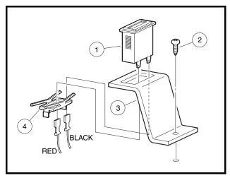
Figure 12-23 Hour Meter Installation
