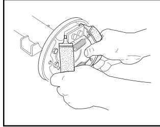
Figure 6-5 Remove Shoe Retainer Clip
