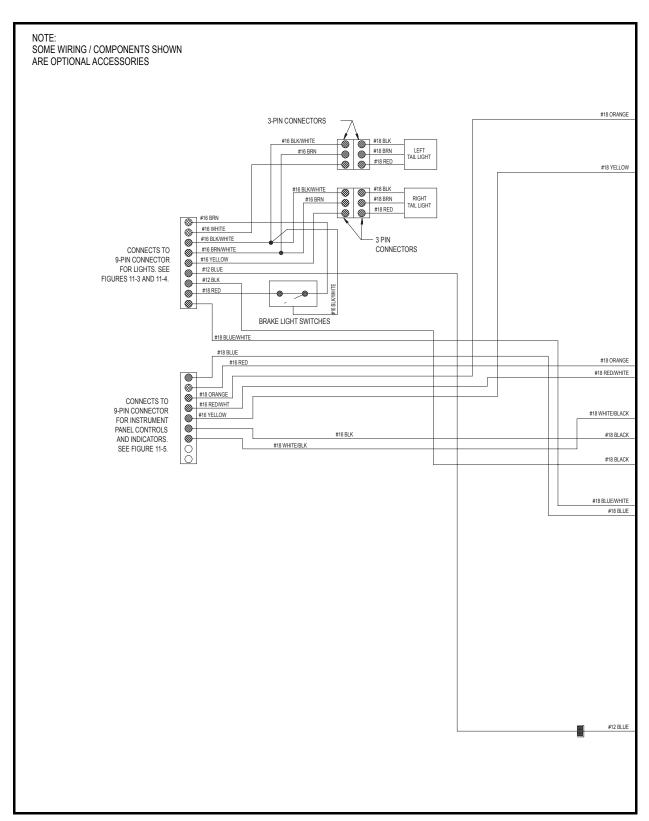
Figure 11-1 Precedent Gasoline Vehicle Wiring Diagram
