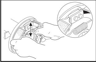
Figure 6-15 Install Leading Shoe
