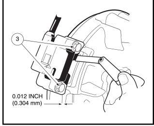
Figure 13-11 Adjust Ignition Coil Air Gap
