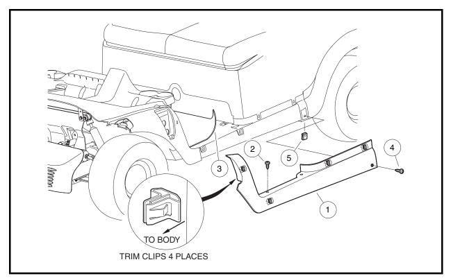
Figure 4-4 Floor Mat Retainer
