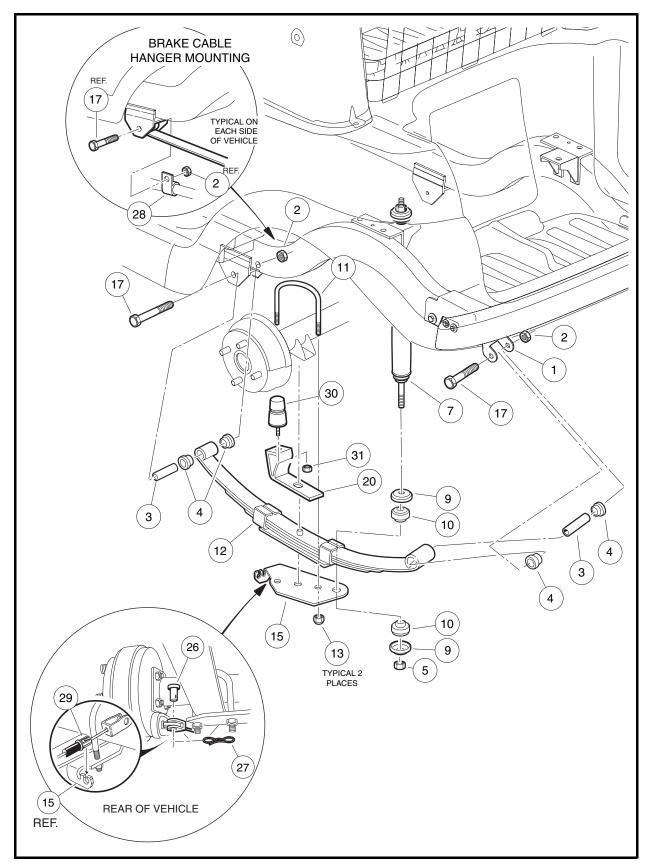
Figure 9-4 Rear Suspension Assembly and Mounting (Four-Passenger Vehicles)
