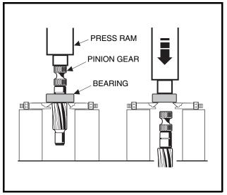
Figure 7-9 Remove Bearing from Pinion
