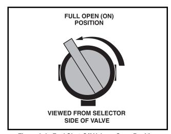
Figure 3-4 Fuel Shut-Off Valve – Open Position
