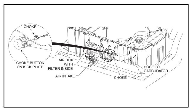
Figure 14-5 Air Intake and Choke Assembly
