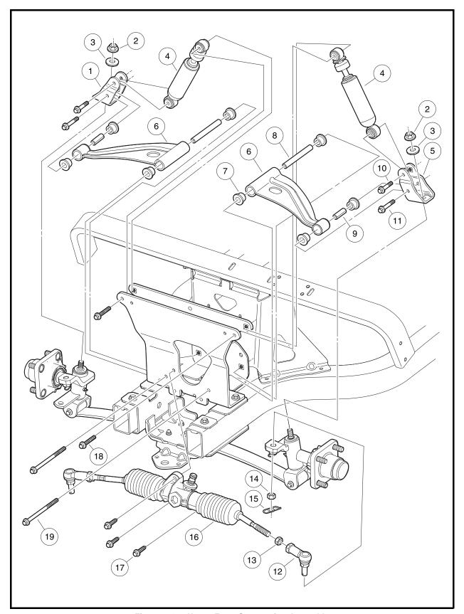
Figure 7-18 Upper Front Suspension Assembly
