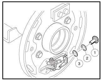
Figure 6-7 Remove Adjuster Wheel
