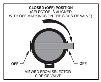
Figure 14-12 Closed Fuel Shut-off Valve Position
