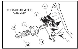
Figure 12-18 Neutral Lockout and Reverse Buzzer
