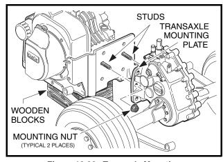
Figure 16-36 Transaxle Mounting
