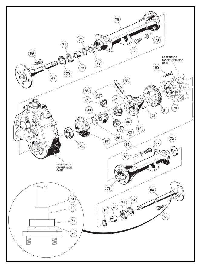
Figure 16-6 Differential Gear Case/Axle Tubes
