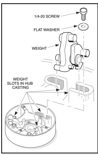
Figure 17-10 Drive Button Mounting
