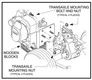
Figure 16-34 Transaxle Mounting
