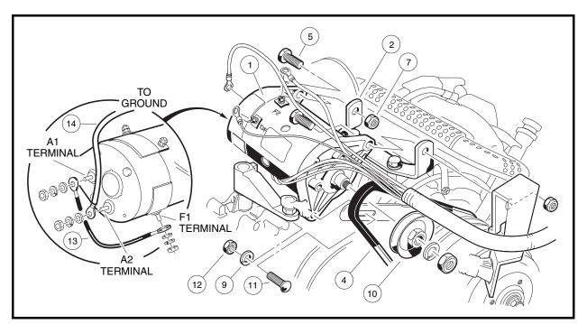
Figure 12-1 Starter/Generator Mounting
