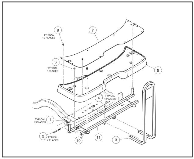
Figure 4-10 Foot Deck (Four-Passenger Vehicles)
