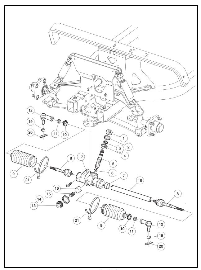
Figure 7-5 Steering Gear
