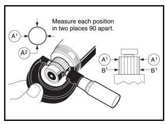
Figure 12-11 Inspect Commutator
