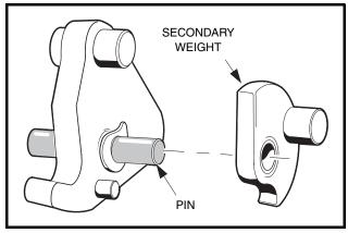
Figure 17-12 Install Pin and Washer
