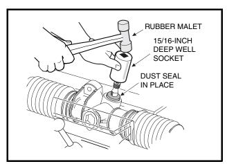
Figure 7-10 Press In Dust Seal
