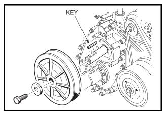
Figure 16-40 Driven Clutch
