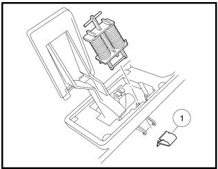
Figure 5-5 Accelerator Spring Clip
