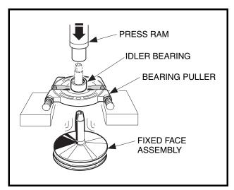
Figure 17-14 Remove Idler Bearing
