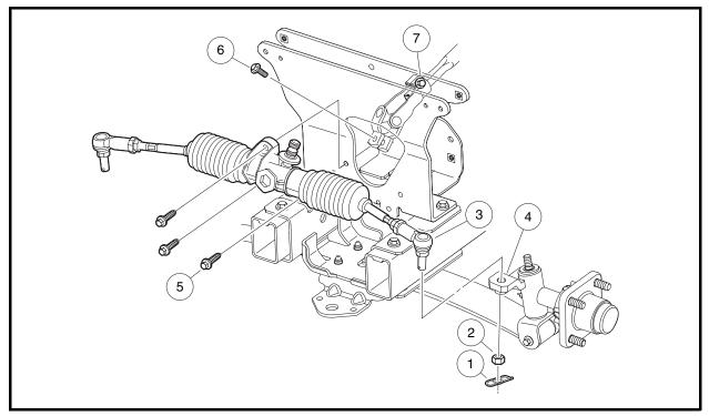
Figure 7-4 Rack and Pinion Removal
