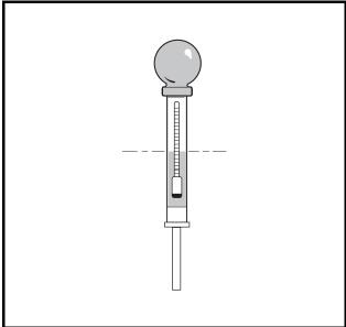
Figure 11-6 Battery Electrolyte Level
