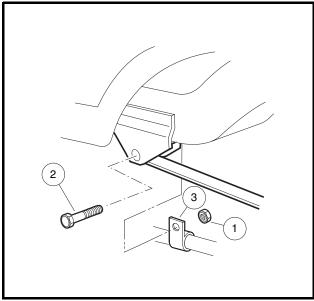
Figure 6-21 Brake Cable Mounting Tab
