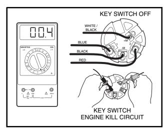
Figure 11-34 Test Key Switch - Engine Kill Circuit
