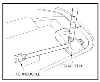
Figure 5-8 Brake Pedal Adjustment
