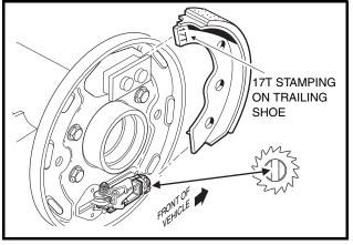
Figure 6-11 Apply Grease To Brake Adjuster
