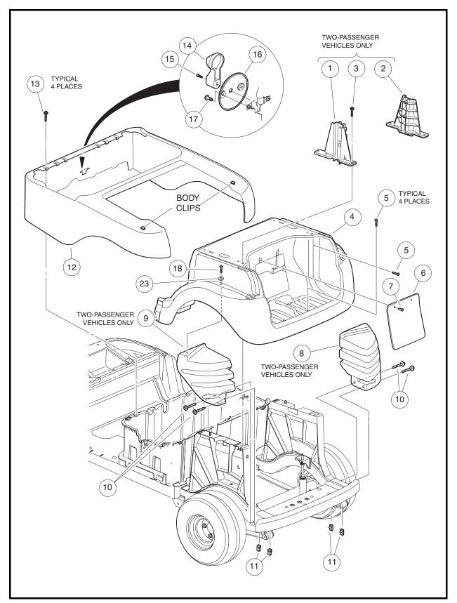
Figure 4-8 Rear Body Components
