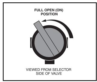
Figure 14-13 Open Fuel Shut-off Valve Position
