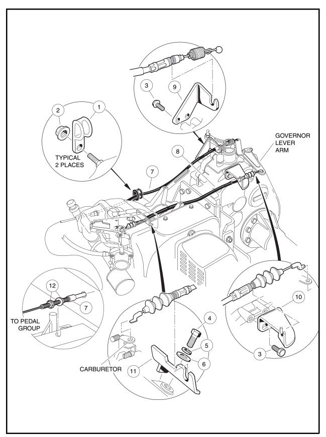
Figure 14-3 Governor and Accelerator Cables
