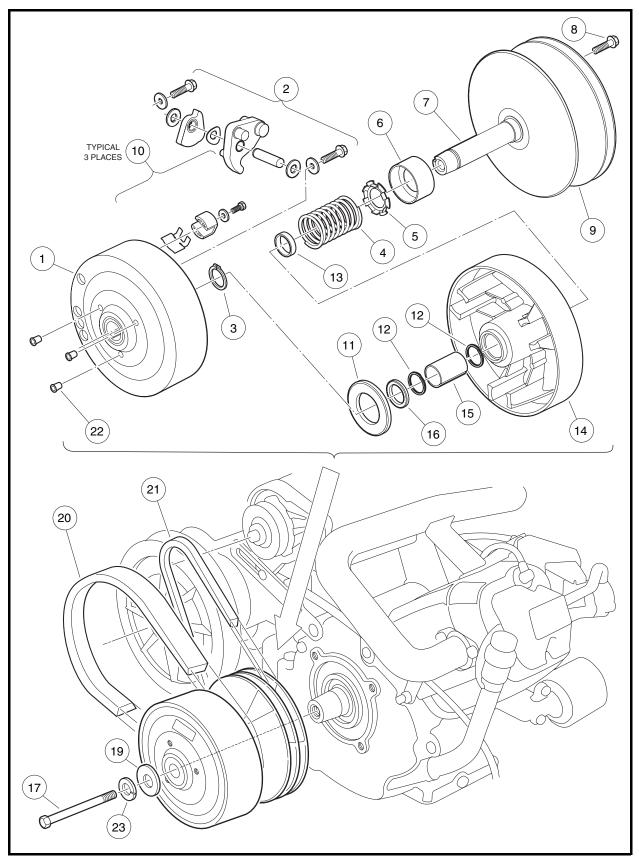
Figure 17-7 Drive Clutch Assembly
