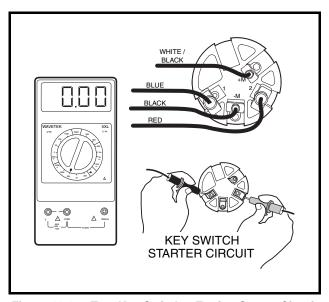
Figure 11-13 Test Key Switch - Engine Starter Circuit
