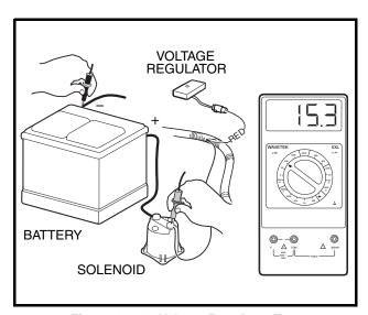
Figure 11-21 Voltage Regulator Test
