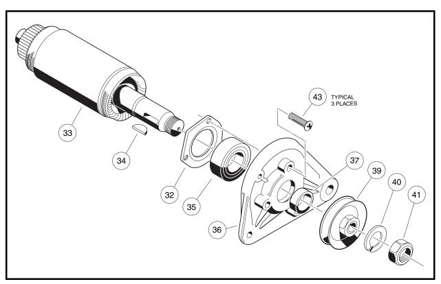
Figure 12-7 Armature and Output End Cover Assembly
