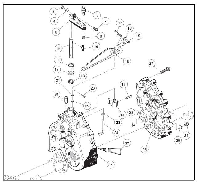
Figure 16-35 Transaxle Gear Casing and Brackets
