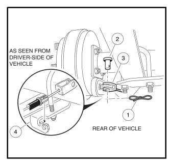
Figure 6-20 Disconnect Cables at Rear Brakes
