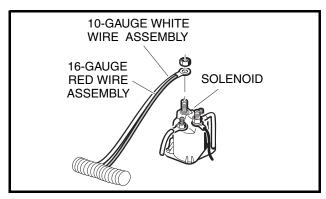
Figure 11-15 Solenoid Wire Removal
