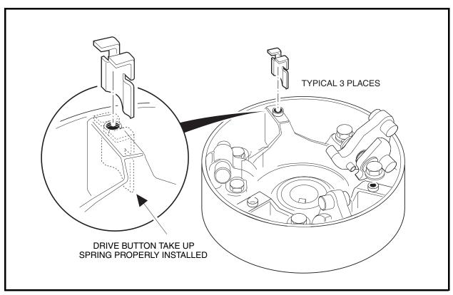
Figure 17-17 Correct Orientation of Drive Button Take-up Spring
