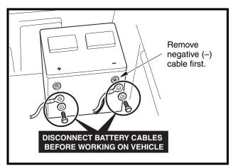
Figure 1-1 Battery Cable Removal
