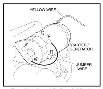
Figure 11-20 Jumper Wire Ground – DF to A2
