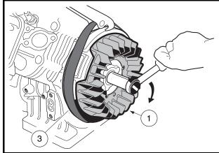
Figure 13-6 Crankcase Cover Installation
