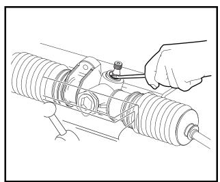
Figure 7-6 Remove Dust Seal
