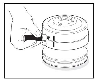
Figure 17-8 Mark Drive Clutch Hub
