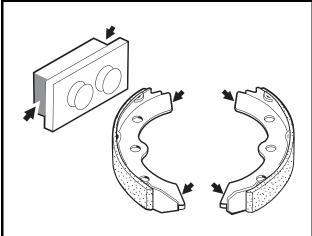
Figure 6-10 Apply Grease To Brake Shoes and Slots
