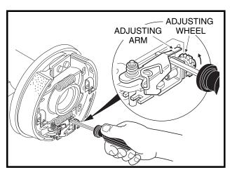
Figure 6-17 Set Adjusting Wheel
