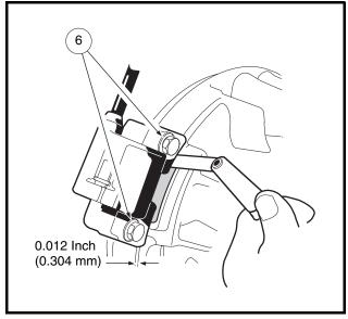
Figure 12-29 Coil Installation
