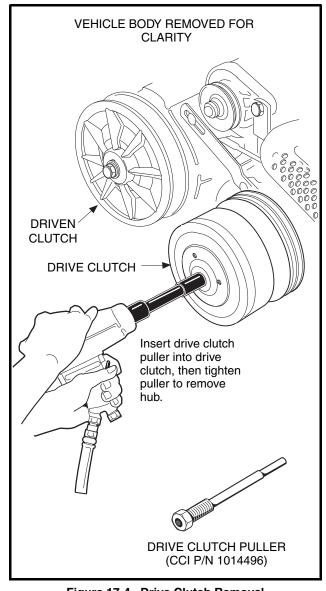
Figure 17-4 Drive Clutch Removal
