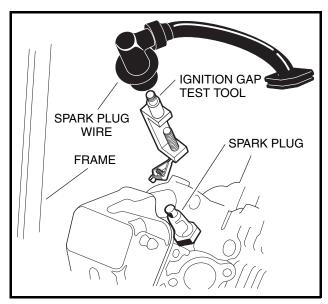
Figure 11-23 Ignition Spark Test
