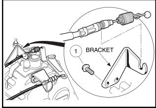
Figure 16-33 Accelerator Cable Bracket
