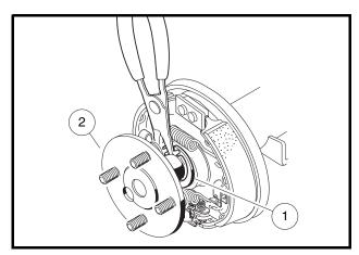
Figure 16-3 Retaining Ring
