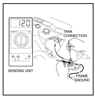
Figure 11-35 Fuel Level Sending Unit Test
