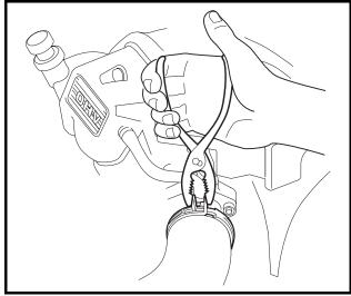
Figure 16-9 Fuel Vent Tube
