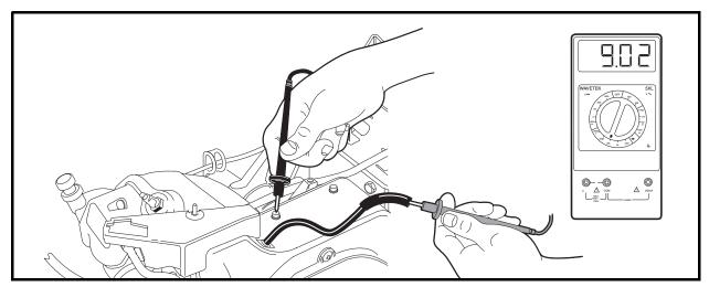
Figure 11-30 Secondary Coil Test without Cap
