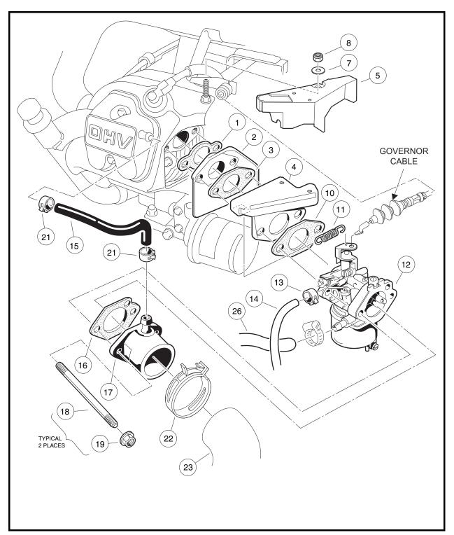
Figure 14-1 Carburetor Installation
