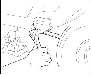
Figure 16-23 Spring Retainer Bolts
