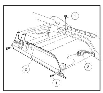
Figure 12-16 Instrument Panel Removal
