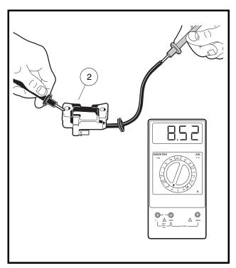
Figure 11-33 Secondary Coil Resistance - Bench Test
