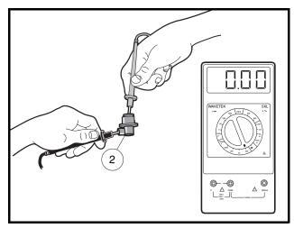
Figure 11-29 Spark Plug Cap Test
