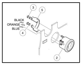
Figure 12-22 Fuel Gauge Installation
