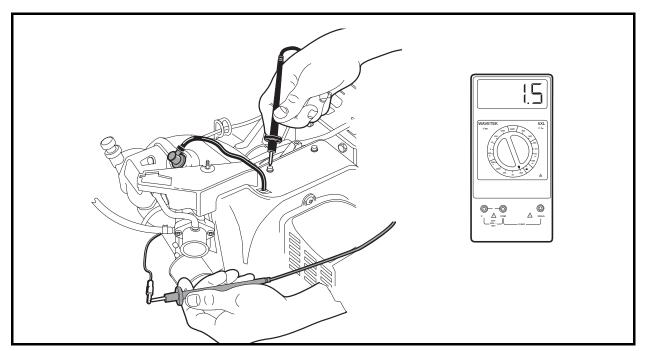
Figure 11-25 Primary Coil Resistance - In Vehicle Test
