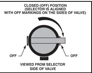
Figure 3-3 Fuel Shut-Off Valve – Closed Position
