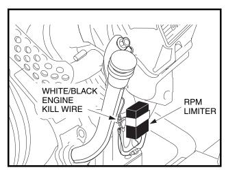
Figure 11-22 Disconnect White/Black Engine Kill Wire
