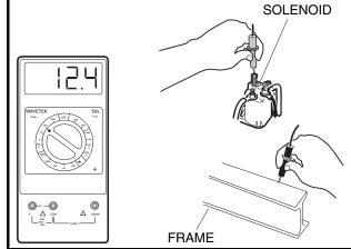
Figure 11-16 Solenoid Continuity Test
