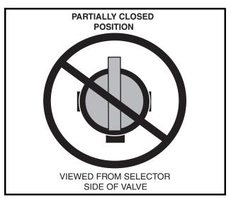
Figure 14-14 Incorrect Fuel Shut-off Valve Position
