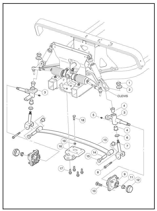
Figure 7-19 Lower Front Suspension Assembly
