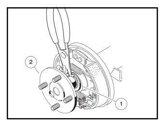
Figure 6-3 Remove Axle Retaining Ring
