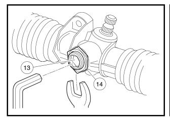
Figure 7-12 Rack and Pinion Adjustment
