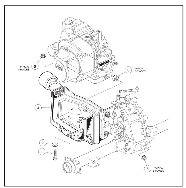
Figure 13-2 Engine Mounting Plate
