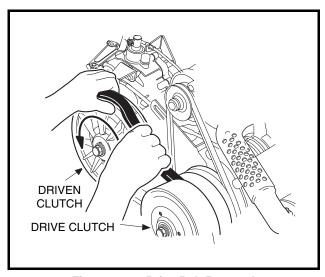
Figure 17-2 Drive Belt Removal
