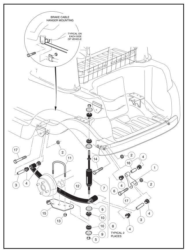
Figure 9-1 Rear Suspension Assembly and Mounting (Two-Passenger Vehicles)
