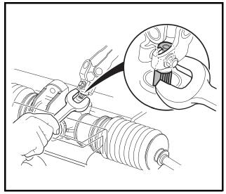
Figure 7-8 Remove Pinion from Housing
