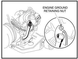
Figure 11-9 Starter/Generator Ground Cable Test
