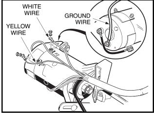
Figure 16-46 Oil Level Sensor Jumper wire
