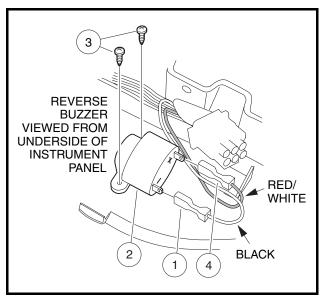
Figure 12-20 Reverse Buzzer
