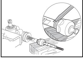
Figure 7-11 Install Ball Joint
