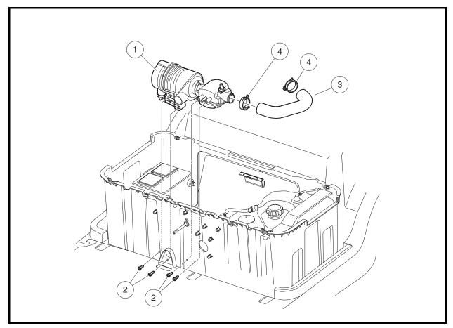
Figure 14-6 Air Intake and Choke Assembly
