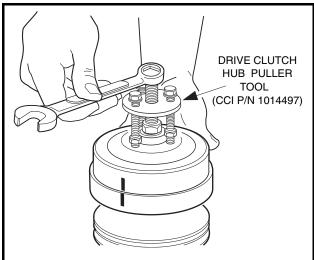
Figure 17-9 Remove Drive Clutch Hub
