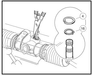
Figure 7-7 Pinion Snap Rings
