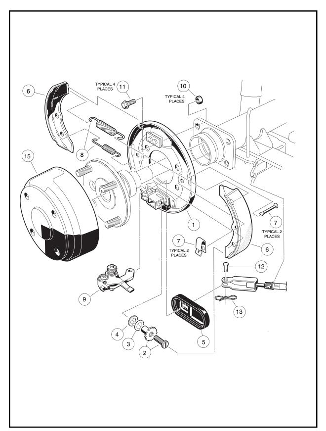
Figure 6-4 Self-adjusting Wheel Brake Assembly
