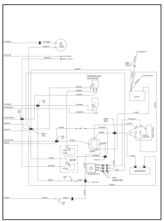
Figure 11-2 Precedent Gasoline Vehicle Wiring Diagram
