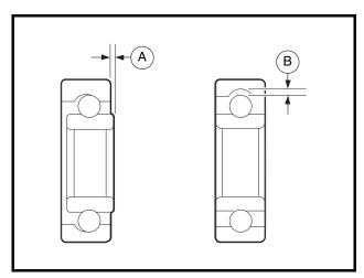
Figure 12-8 Bearing Play Inspection
