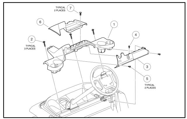
Figure 4-3 Instrument Panel
