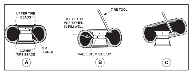
Figure 8-1 Tire Removal
