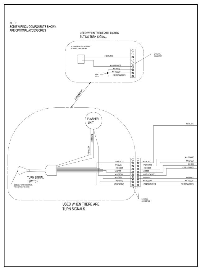
Figure 11-3 Precedent Gasoline Vehicle Accessory Wiring Diagram (Optional)
