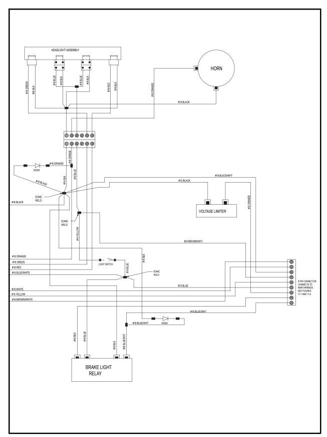
Figure 11-4 Precedent Gasoline Vehicle Accessory Wiring Diagram (Optional)
