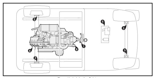
Figure 11 Lubrication Points
