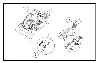
Figure 13-13 Check Engine Oil Level
