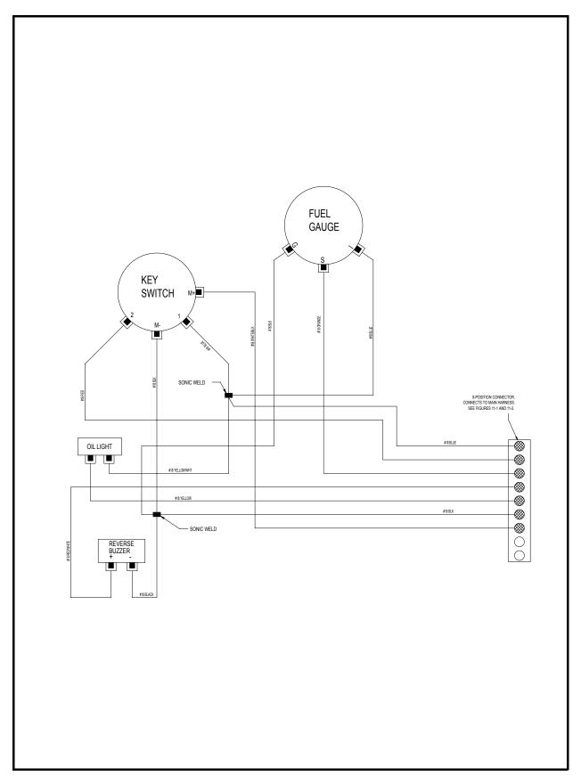
Figure 11-5 Precedent Gasoline Vehicle Instrument Panel Wiring Diagram
