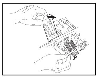
Figure 5-7 Accelerator Spring Pin Removal
