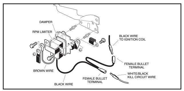
Figure 12-24 RPM Limiter Assembly
