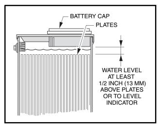
Figure 12-31 Battery Water Level
