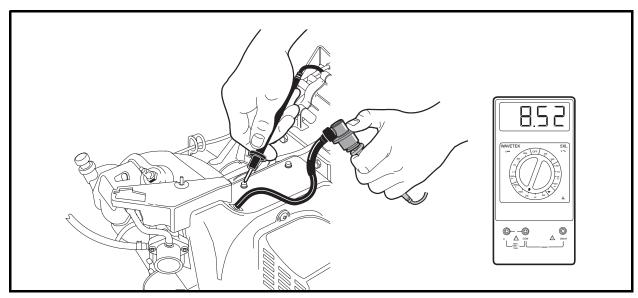
Figure 11-26 Secondary Coil Test - In Vehicle Test
