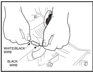
Figure 16-17 Oil Level Sensor Jumper Wire
