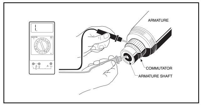
Figure 12-12 Armature Ground Test
