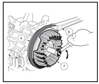
Figure 13-10 Flywheel Nut Removal
