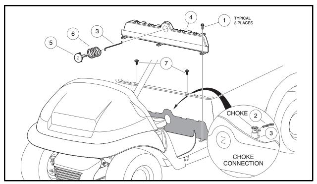
Figure 4-5 Kick Plate and Choke Button
