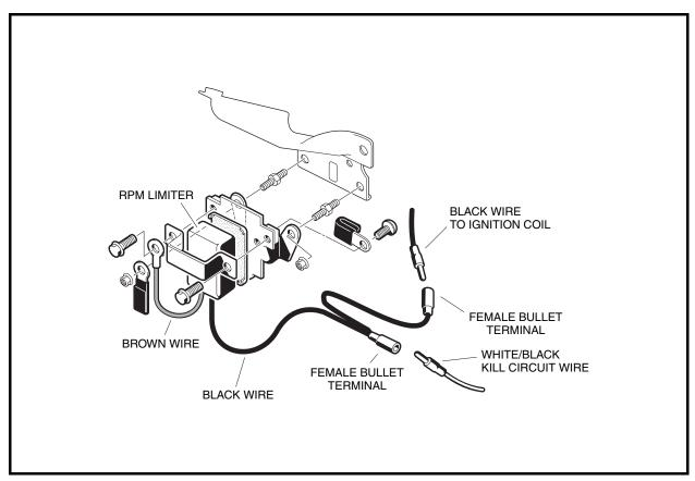
Figure 11-24 RPM Limiter
