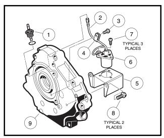
Figure 13-5 Oil Level Sensor
