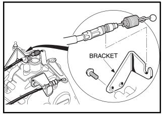
Figure 16-37 Accelerator Cable Bracket
