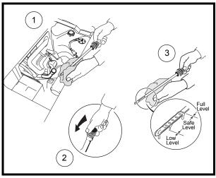
Figure 10-1 Engine Oil Level Check
